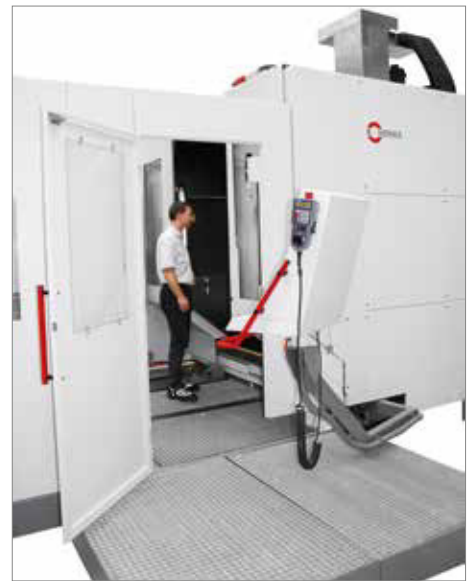
Side access to the working area of the C 52 U for manual operations or in setup mode.
