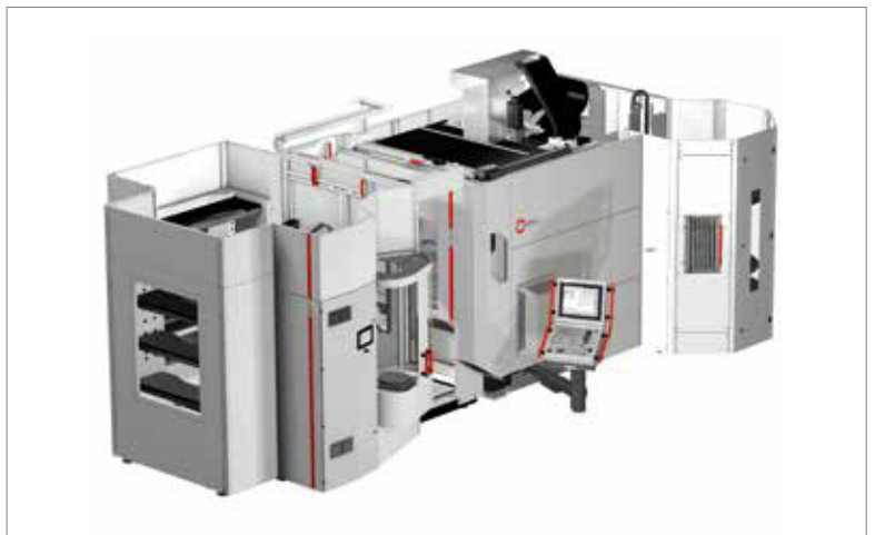
HS flex with two pallet storage moduls and setup station, adapted on a machining centre C 42 U.
