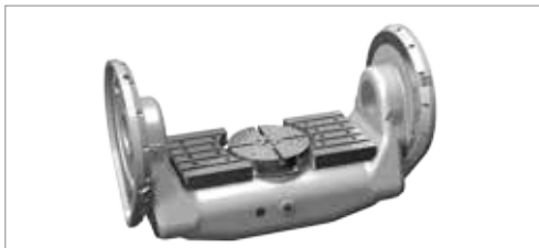
Secondary clamping plates . 760 x 370 mm
