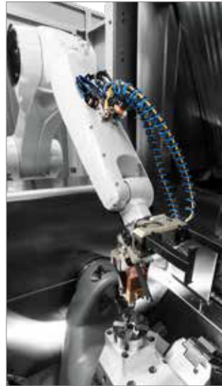
Loading a workpiece using the robot
