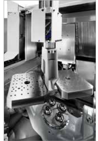
Double gripper for 2 x 100 kg
