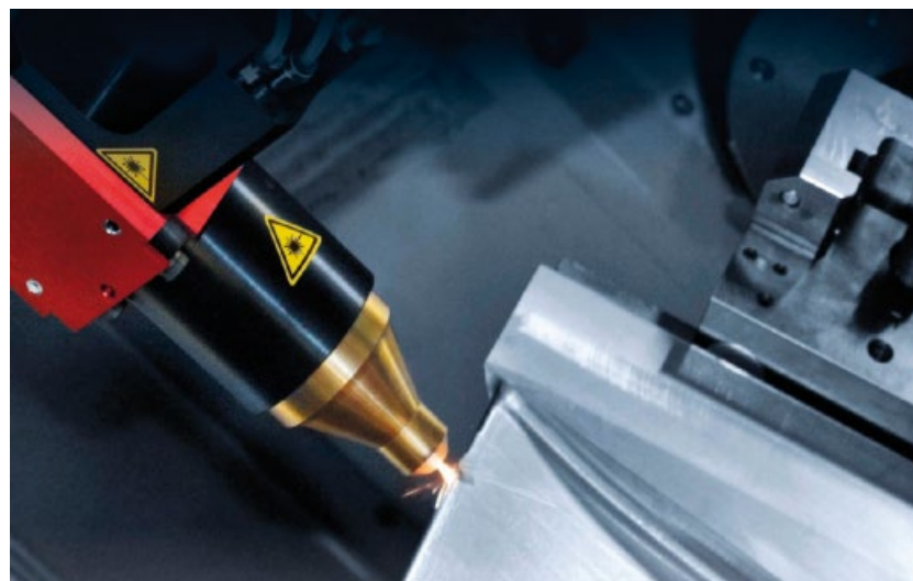
Fig. 3 Laser cladding head in operation on a turbine blade
