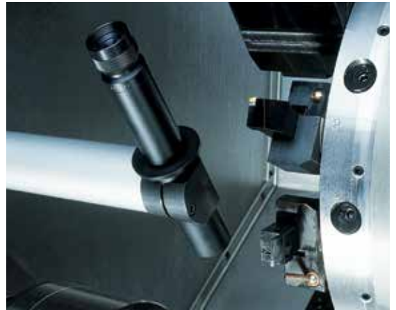
Automatic tool position calculation forms part of the basic equipment – TRAUB ATC.
